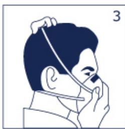
Place the top band high on the back of your head. Move the bottom band over your head and position it below your ears.
